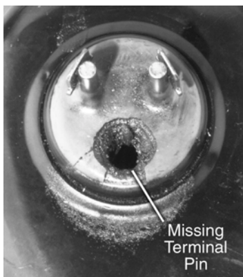
Figure 1-3. Close-up view of hermetic terminal after it has vented.
