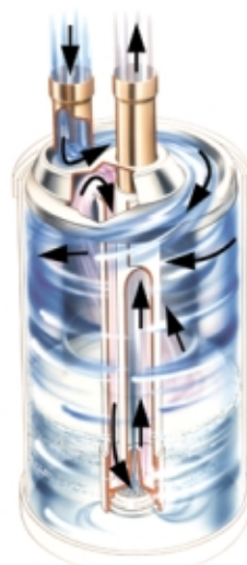
Figure 6-14. A suction line accumulator prevents damaging liquid refrigerant floodback.
